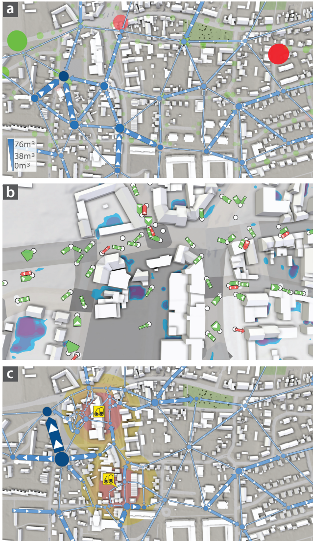
Figure 6: Flow maps for storm water. (a) Overview. Circles indicate the sewer effects (red=outflow, green=inflow). (b) Glyphs show details about the sewer-surface coupling. (c) Increased local LoD nearby important buildings.
